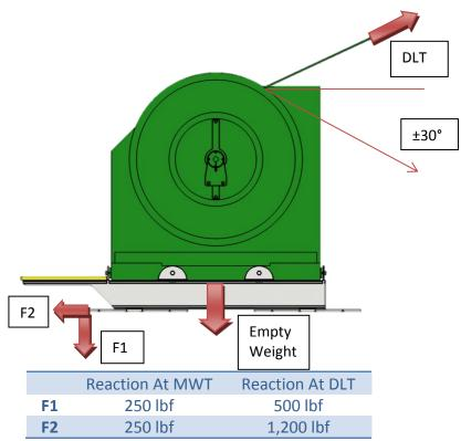
Forces are maximum forces per bolt, at DLT, for a 16 bolt hold down pattern (Rows spaced at 24", 48", and 72"). Analysis is good for a vertical fleet angle of  $\pm 30^{\circ}$  and a horizontal fleet angle of  $\pm 5^{\circ}$ .
